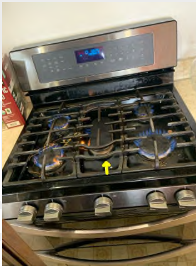
Middle burner not fully igniting
